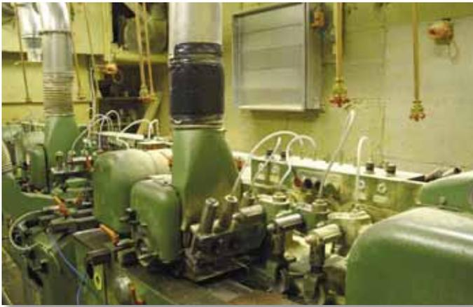
Firefly's PlanerGuard monitors this type of machine by using *flame detectors monitoring the open area*. It is important that extinguishing can take place even in closed areas of the planer. This is especially true for open planers. *Water mist* will extinguish fire quickly and efficiently, even in these closed areas. Water mist also ensures that your planer isn't damaged by water.
